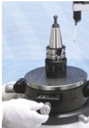
Manual part alignment via digital micrometers
