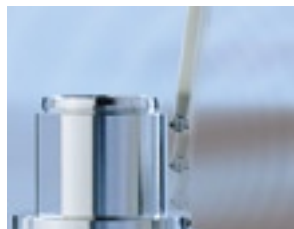
Cylindricity measurement via vertical spiral trace
