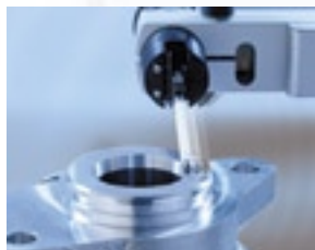
Flatness measurement via horizontal spiral trace
