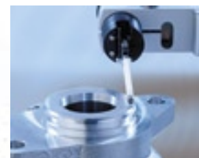
Flatness measurement outside, horizontal
