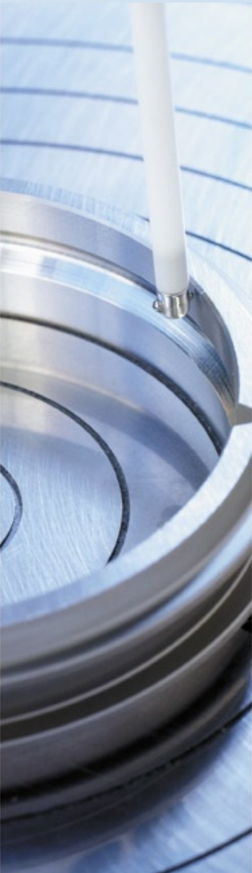
Cylindricity measurement via vertical spiral trace
