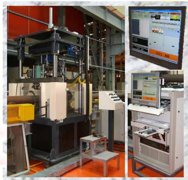
DTB-800A (Full automatic measuring system for Brinell hardness)
